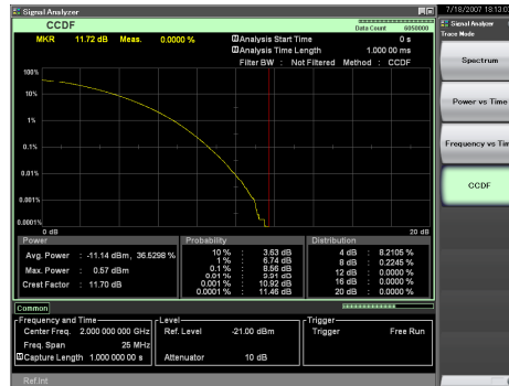
Screen: CCDF Analysis (W-CDMA, TestModel1 64DPCH x 4 Carrier, 2 GHz)
