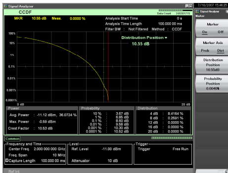
Screen: CCDF Analysis (W-CDMA, TestModel1 64DPCH, 2 GHz)
